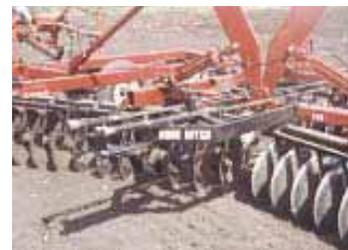
“Sure Hitch” clamps onto a toolbar and consists of a spring-loaded pin, guide assembly, and drawbar. Drawbar can be pulled backward 15 in. and swung 15 in. from side to side.
