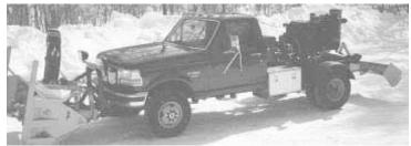
Pickup is equipped with 7 1/2-ft. snowblower on front and 6 1/2-ft. snow blade on back.
