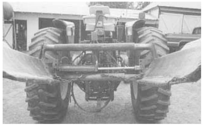
Handler consists of a pair of 44-in. long hydraulically operated steel arms.
