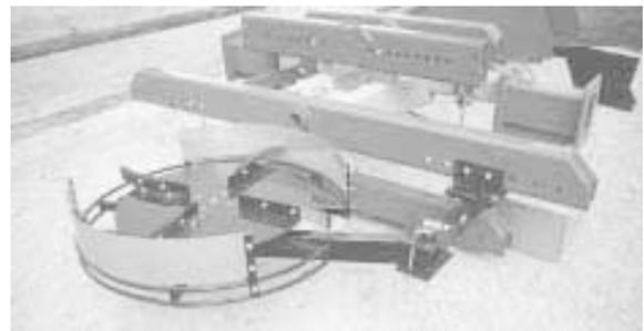
Hydraulic-driven spreader mounts on steel swing arm.
