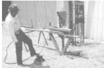
walled pipe. He attached a ring to the top of the press so he can pick it up with a tractor loader to move it. He says there's nothing on the market like it that's priced reasonable and he built it mostly out of scrap parts. (C.F. Marley)
