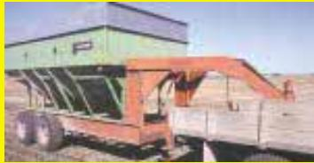
The rig consists simply of a 450-bu. capacity Parker Brothers wagon mounted on the gooseneck trailer frame.
