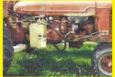
First, we changed the pto from the rear to the right side. We did so by removing the belt pulley and installing a splined pto shaft in its place. This way it's easier to connect to the 10-in. dia., 22-ft. bin unloading auger we use.
