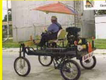
Powered by an 18 hp Vanguard engine coupled to a 3-speed differential out of an old Ford riding mower, it has a top speed of 6 1/2 to 7 mph.
