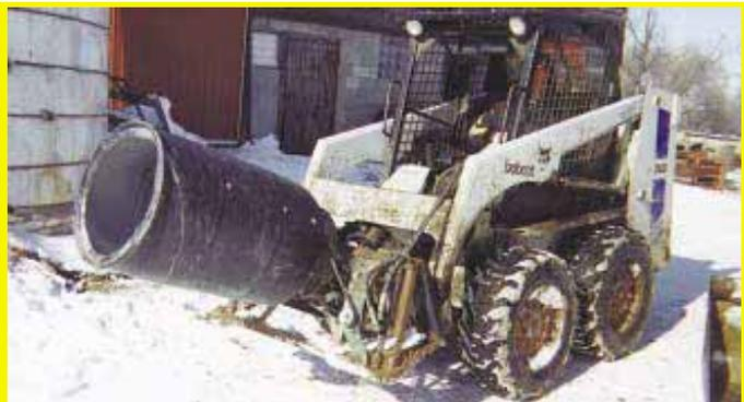
Using a 50-gal. barrel I built a cement mixer that quick taches to my Bobcat skid steer loader. Paddles bolt to the inside of the barrel to mix the cement. The orbit motor (salvaged from an old combine) runs off skid steer hydraulics. To mount the barrel I used the spindle off an old wagon running gear. I left the wheel rim on and bolted the barrel to the edge of the rim. I used three pieces of 2 1/2-in. angle iron to make the paddles.
