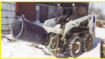
Using a 50-gal. barrel I built a cement mixer that quick taches to my Bobcat skid steer loader. Paddles bolt to the inside of the barrel to mix the cement. The orbit motor (salvaged from an old combine) runs off skid steer hydraulics. To mount the barrel I used the spindle off an old wagon running gear. I left the wheel rim on and bolted the barrel to the edge of the rim. I used three pieces of 2 1/2-in. angle iron to make the paddles.
