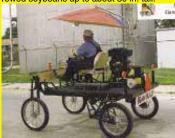
Powered by an 18 hp Vanguard engine coupled to a 3-speed differential out of an old Ford riding mower, it has a top speed of 6 1/2 to 7 mph.
