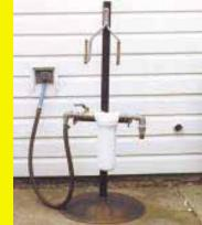
pipe stand. I made the stand by welding a 3ft. long, 3/4-in. dia. steel pipe into the center of a 2-ft. dia. disc.
