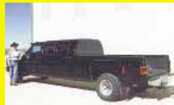
crew cab pickup to the back half of a 1984 Chevy 4-door crew cab pickup. I bought the 1991 model at a city auction and cut it through the middle of the back doors. I bought the 1984 model at a wrecking yard and cut it through the middle of the front doors. I hired a welder to beef up the frame and lengthen it an additional 38 in.
