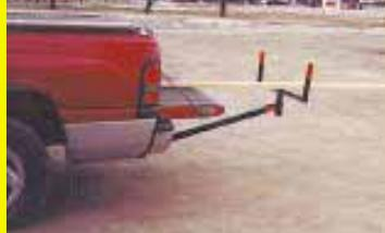
and is also adjustable in height. Orange plastic caps slide over the top of the vertical side posts to make the unit more visible. Folds for storage in the back of the pickup, inside a toolbox, etc.
