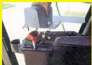
kids from accidentally activating the controls. It consists of sheet metal formed to cover all the controls on the console and a keyed latch to hold it securely in place. Padding on the bottom side prevents scratching. I lock the cover in place whenever getting out of the cab, especially when small children are around. (Eric Schmidgall, 33652 Townline Rd., Mackinaw, Ill. 61755 ph 309-392-2322)
