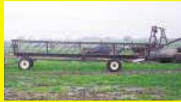
ules so the trailers are available cheap. The axles are 16 ft. apart with 24-ft. long beds that are 2 ft. deep and 4 ft. wide at bottom. They're 7 ft. wide at the top.
