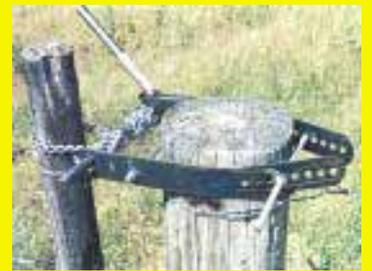
and stretch them tight. It consists of two strap iron brackets that clamp over the post with two long bolts. Fits over any post from 6 to 11 in. dia. It costs a lot less to set up a gate this way than with solid gate panels. Our clamp-on model sells for \$24.95; bolt-on model for \$22.95. **(Jim Circle, 1090 30 Rd., Woodston, Kan. 67675 ph 785-994-6278)**
