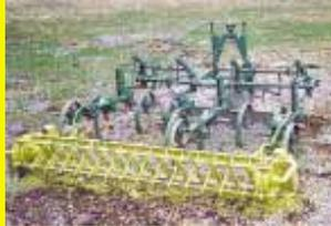
spikes that hold it all together. The combination of spikes and cross bars breaks up clods. It hinges up and down on brackets behind a Deere model B cultivator. I use the whole rig as a field harrow and it really digs well. **(Tom Kutruff, Rt. 1, Box 37, Altoona, Penn. 16601 ph 814 944-9205)**
