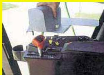
kids from accidentally activating the controls. It consists of sheet metal formed to cover all the controls on the console and a keyed latch to hold it securely in place. Padding on the bottom side prevents scratching. I lock the cover in place whenever getting out of the cab, especially when small children are around. **(Eric Schmidgall, 33652 Townline Rd., Mackinaw, Ill. 61755 ph 309-392-2322)**
