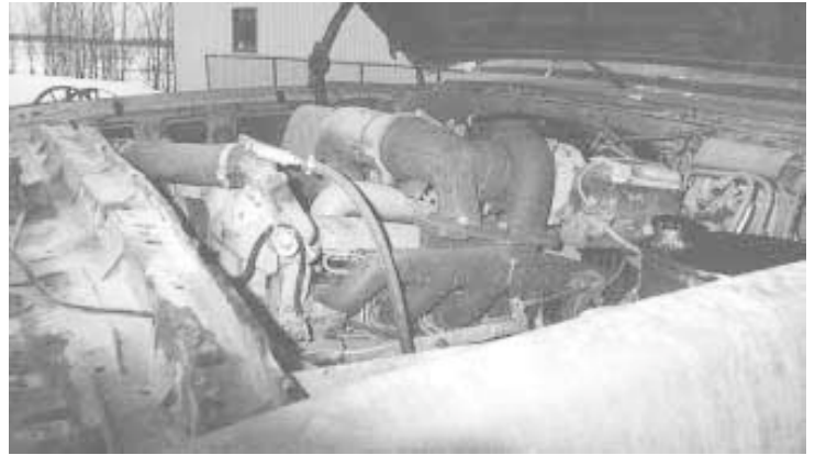
Pickup was repowered with a 359 cu. in., 6-cyl. diesel engine out of a Deere industrial loader. Gerber didn't want to make a "bubble" in the hood so he raised the entire cab.
