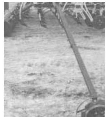
An orbit motor "telescopes" marker out to its full working length.
