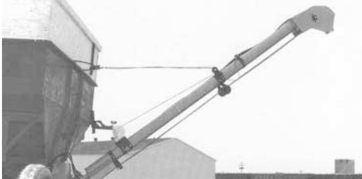
Conveyor belt, which is 8 in. wide, is enclosed in a 6-in. dia., 15-ft. long auger tube.
