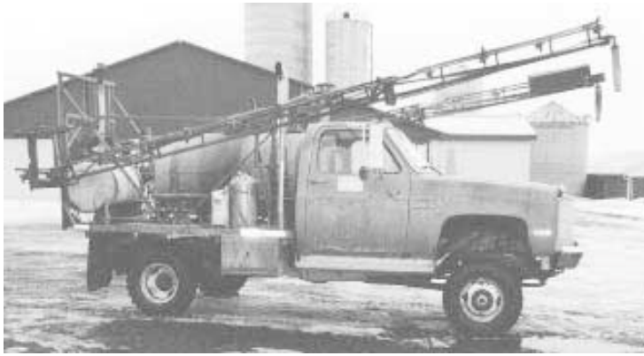
Gerber's repowered 4-WD pickup is equipped with a 50-ft. sprayer and 500-gal. tank. 1-TON CHEVY REPOWERED BY 200 HP DIESEL
