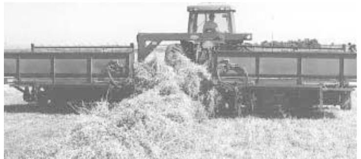
New swath turner is equipped with a pair of 8-ft. wide belt pickups and 11-ft. wide draper tables that gently handle hay.
