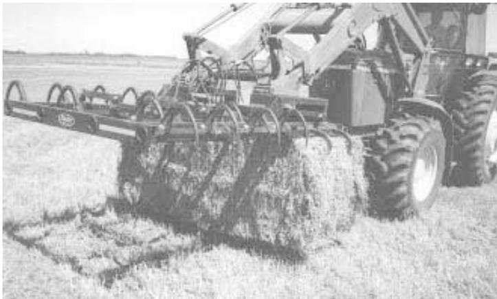
Bale grab is equipped with three sets of teeth, and electric/hydraulic controls that allow each bale to be loaded or unloaded independently.
