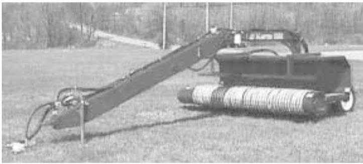
Inverter is equipped with a 12-ft., 6-in. wide pickup drum that rakes or merges windrows without driving over the crop.
