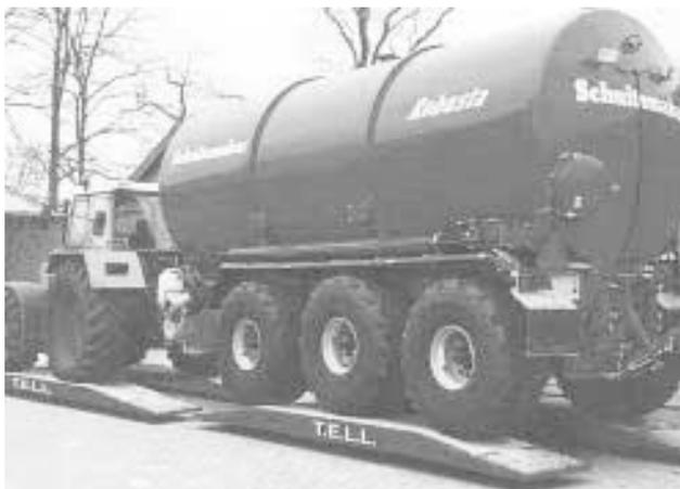
Portable scale can weigh tractor-wagon combinations up to 60 ft. long, depending on how it's laid out, and can weigh loads up to 80 tons.
