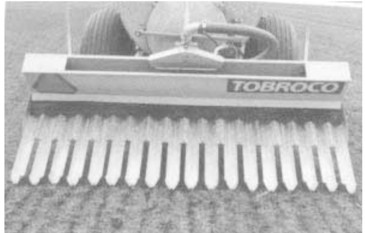
Manure flows through a hose to a trough fitted with a row of angled downspouts. Each downspout is fitted with a knife on the bottom that cuts a slot for manure to flow into.
