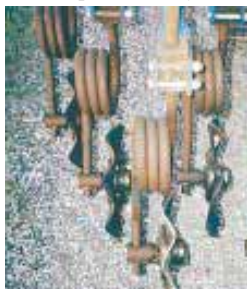
Coulters can be mounted in any configuration with both left and right hand models available.
