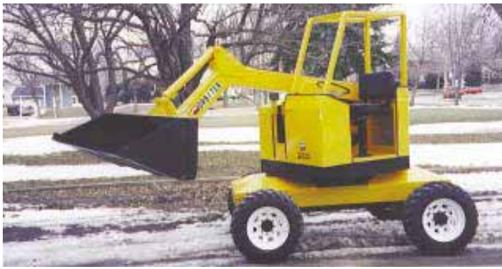
New loader tractor is equipped with a turret that rotates 360 degrees.
