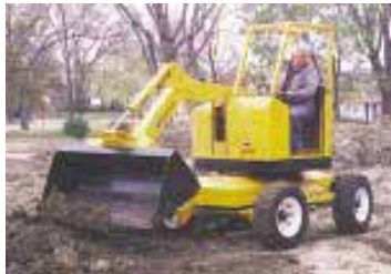
Rotating turret lets you scoop up a load in front and dump it to the left or right without moving the tractor.
