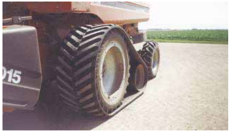
"Fargo Tracks" are 30-in. wide rubber tracks that fit over standard size (42-in.) dual wheels equipped with a 24-in. steel idler wheel. To mount the tracks you remove the combine's original wheels and install the company's customized duals.
