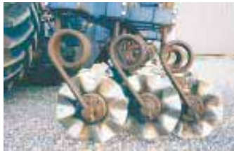
The 17-in. dia. coulters are arranged in three rows. Each coulters ride on a spindle supported by an 18-in. long coil spring stem that clamps onto caddy toolbar.
