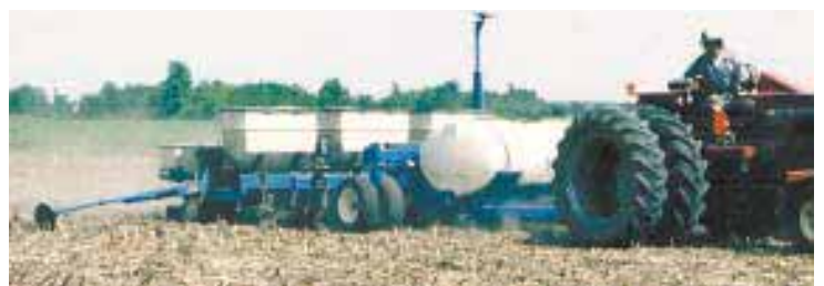
McIlhargey uses the coulters on a home-built no-till coulters caddy. It carries a 500-gal. liquid fertilizer tank and is pulled in front of a 6-row double frame Kinze corn planter.
