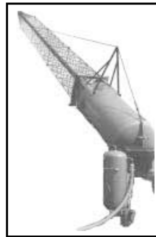
Cannon fires pumpkin with compressed air from a 1,500-gal. air tank.
