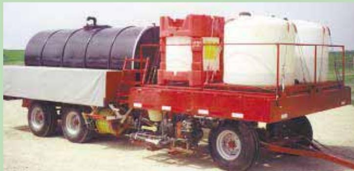
Trailer is built on the chassis of an old pull-type pea harvester. It’s equipped with a slide-out pump, inductor and hoses that Kennay can easily reach from the ground.
