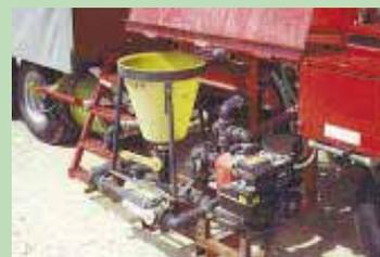
Chemical tanks are plumbed to 15-gal. inductor, which mounts on a slide-out shelf under the tanks along with a 5 hp pump.
