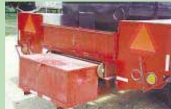
Roll-out metal parts box on back is used to carry extra spray nozzles, pump diaphragms, etc.
