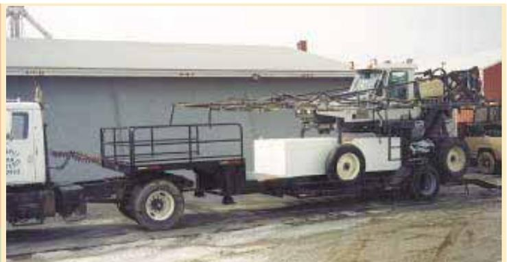
Gooseneck trailer is equipped with an upper and lower deck and was designed to carry a Melroe sprayer. Loganbill pulls it with an International single axle semi tractor.
