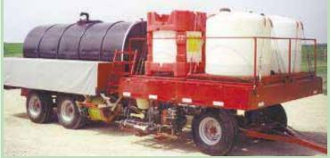
Trailer is built on the chassis of an old pull-type pea harvester. It's equipped with a slide-out pump, inductor and hoses that Kennay can easily reach from the ground.
