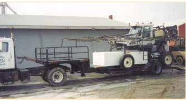
Gooseneck trailer is equipped with an upper and lower deck and was designed to carry a Melroe sprayer. Loganbill pulls it with an International single axle semi tractor.
