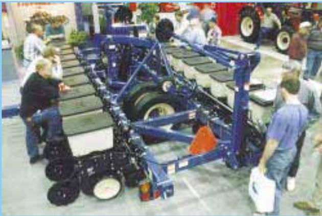
**Kinze introduced this first-of-its-kind planter at the recent Farm Machinery Show in Louisville. Transport wheels are tucked in between front and rear toolbars, allowing row units to be spaced as close as 10 in. together.**
