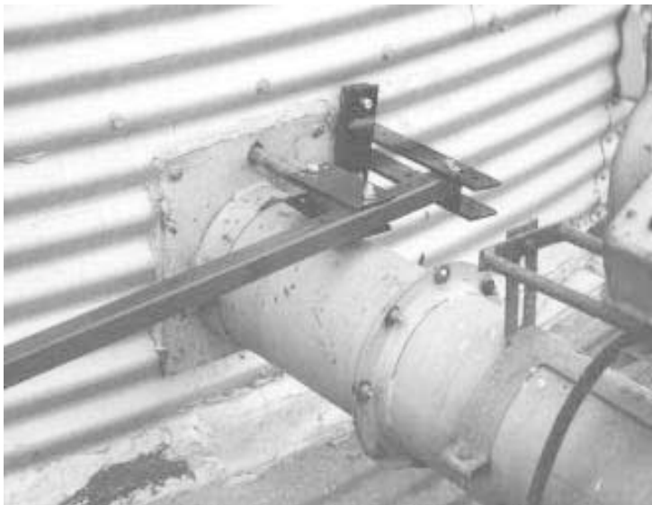
To open grain well, you simply pull on the 4-ft. handle, which provides leverage.
