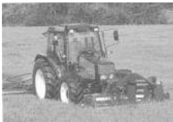
Valmet bi-directionals run at speeds of up to 25 mph in either direction with a full 3-pt. hitch and pto on each end.
