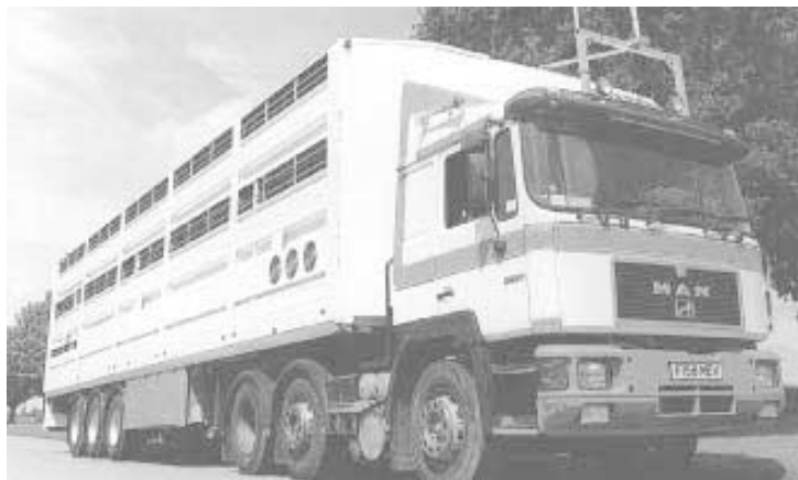
Researchers built this ventilated trailer in response to animal welfare concerns.
