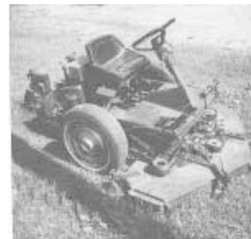
Three-wheeled mower is built around a car axle.
