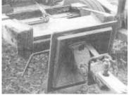
To hook up applicator to tank you pull the winch cable out through the receiver hitch, hook up to the drawbar, and pull it in.
