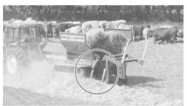
Single flow control valve lets you adjust speed of auger so you can precisely control the amount of grain deposited on windrow.
