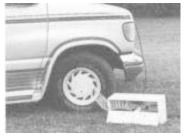
Compressor is oil-less for low maintenance and is 100 percent duty cycled so you could run it for 24 hours a day with no problems, if necessary.
