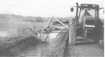
Spring-loaded equalizer allows cleaning head to be guided by the ditch walls and gives the operator a 15 in. lateral drift and 8 in. vertical free movement.
