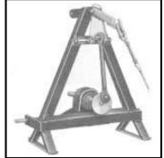
A-shaped 3-pt. mounted frame with a bearing-mounted pto shaft hooks up to tractor pto.
