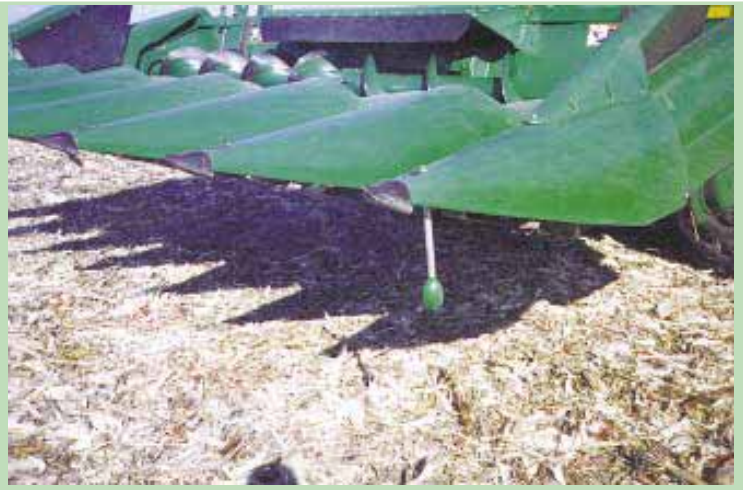
Sensor fits directly under the front point and consists of a spring-loaded arm that follows the ground contour. It's wired to a control box that also mounts on the head.
