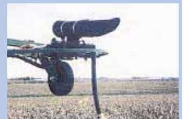
Cameras mount over spray markers at each end of boom. System comes with its own power supply unit.
