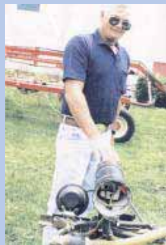
Boom-mounted cameras mount inside protective housings made from specially-shaped PVC Tubes.
