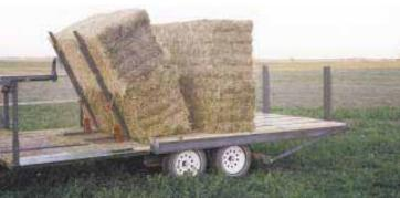
A pair of forks, recessed in deck, push pairs of bales backward on trailer's rear deck.
