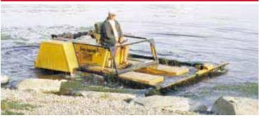
"Sea Horse" has a 12-ft. wide sicklebar on front that can be lowered hydraulically to a maximum depth of 7 ft. A wire mesh basket collects the clippings.
