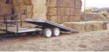
Once both decks are fully loaded, the rear deck is tilted backward and the bales slide off in a row ready for stacking.
