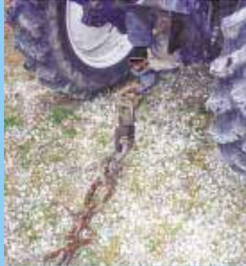
Drawbar clevis is fitted with a pair of swivel hooks, allowing chain to tumble as it rolls along.
