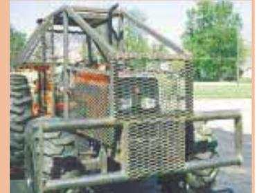
Cage includes "push bars" up front and a protective grille so Knepler can drive right over small trees and brush.
