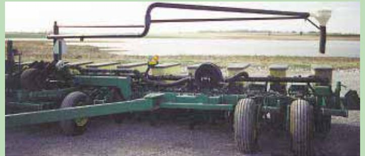
Planter-mounted "air boom" swings across full width of planter and is designed to be used together with any pneumatic seed blower or grain vac.
