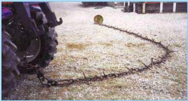
The 15-ft. length of log chain is "spiked" with 8-in. long steel crossbars welded on at 6-in. intervals. A "wheel rim" weight keeps chain tight so that it stays in contact with soil.
