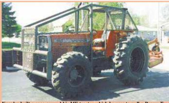
Knepler built a cage around his MF tractor which he uses to pull a Brown Tree Cutter. The pto-powered chopper-mower pushes over trees and cuts them up.
