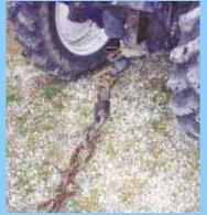
Drawbar clevis is fitted with a pair of swivel hooks, allowing chain to tumble as it rolls along.
