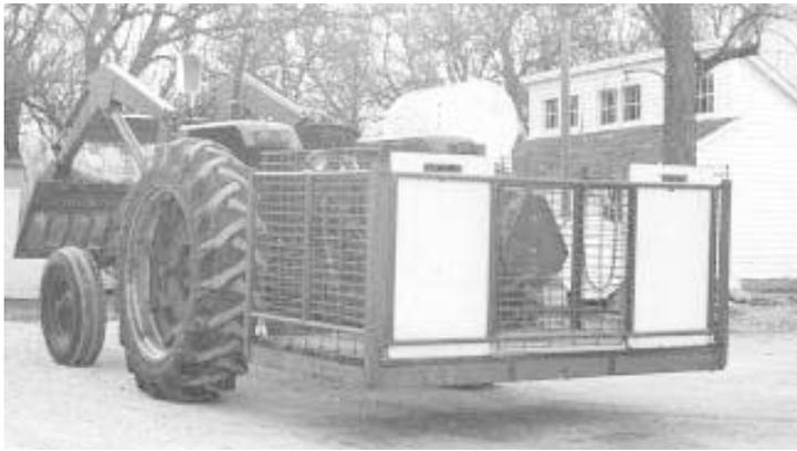
A pair of sliding wooden doors on each side of the trailer are raised to let hogs in or out.
