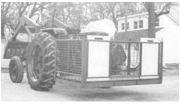
$\label{eq:Apair} \textbf{A pair of sliding wooden doors on each side of the trailer are raised to let hogs in or out.}$
