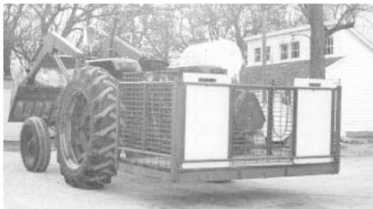
A pair of sliding wooden doors on each side of the trailer are raised to let hogs in or out.
