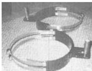
“Saddles” are made out of 2-in. wide strips of 10-ga. steel pipe and straps are 7-in. dia. hose clamps.
