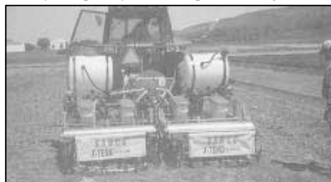
Experimental planter from Ireland has been used by the Center for Plasticscience to plant corn under a layer of plastic. The plastic disappears by season's end.
