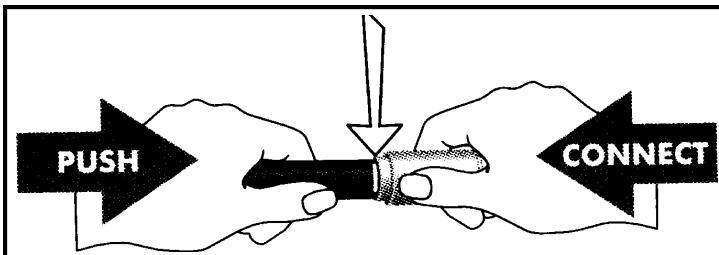
Fittings can be attached to the company's special thermal plastic hose by hand.
