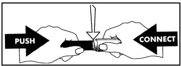
Fittings can be attached to the company's special thermal plastic hose by hand.
