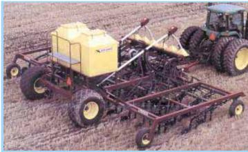
Scheetz says his 40-ft. Seed Hawk no-till air seeder plants crops in rows as narrow as 12 in. without plugging up. Seed and fertilizer are augered to meters up front.
