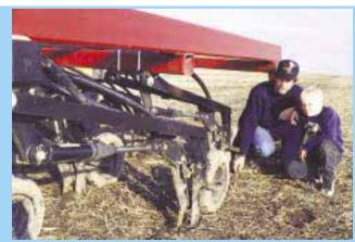
Each row unit mounts on a 7-ft. arm fitted with a hydraulic cylinder. Cylinder applies downpressure to a pair of 1/2-in. wide "fracturing knives" that place seed and fertilizer in ground with minimal sidewall compaction.
