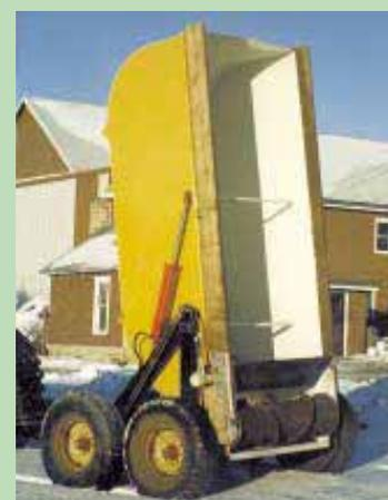
Spreader is raised and lowered by 4-in. hydraulic cylinders mounted on each side. It raises straight up to vertical to completely empty out all of the material.
