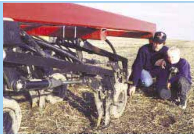
Each row unit mounts on a 7-ft. arm fitted with a hydraulic cylinder. Cylinder applies downpressure to a pair of 1/2-in. wide "fracturing knives" that place seed and fertilizer in ground with minimal sidewall compaction.
