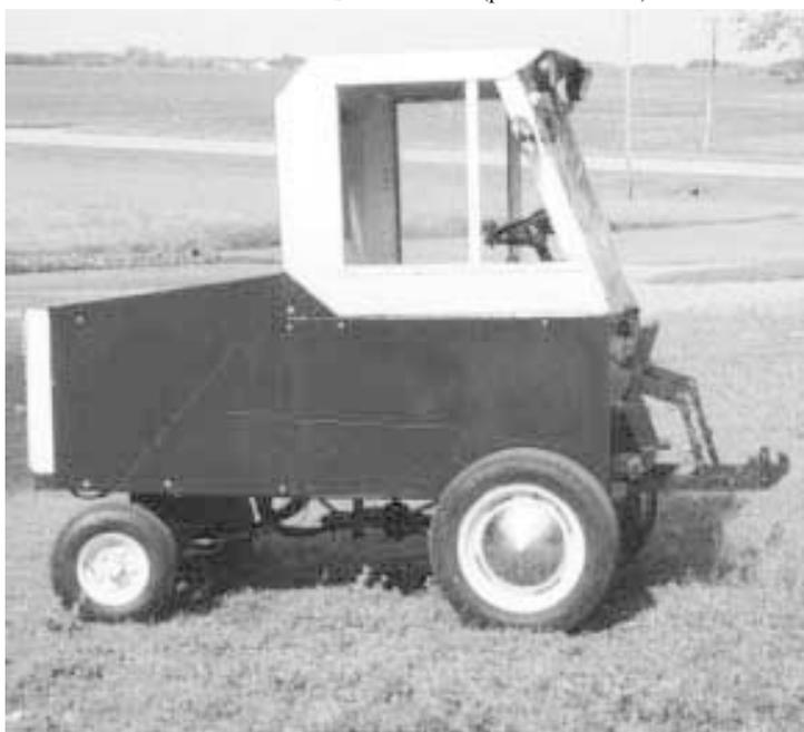
**The 2-WD rig has a cab as well as a 3-pt. hitch and pto on front. Fisher used the bean rider's engine, seat, hydrostatic transmission, live hydraulics, power steering, fuel and hydraulic tanks, hydraulic hose, and battery.**
