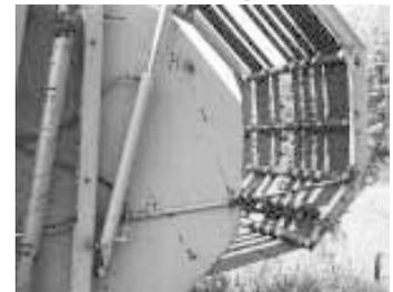
"I designed a pair of safety arms for my Vermeer 605C round baler. The problem is when hay wraps around the rollers and belts the only way to unplug it is to stand inside the baler with the back open. If a hydraulic hose breaks or someone touches the controls, the back can slam down on the person unplugging the machine.
