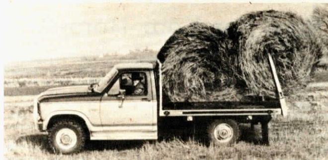
Hydra-Bed will pick up, haul and unroll two bales weighing up to 2,100 lbs. each.
