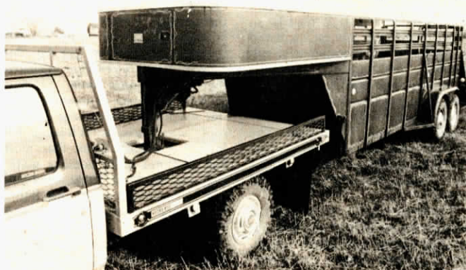
Recessed well allows gooseneck trailer to be hooked up without interfering with the bale loader.
