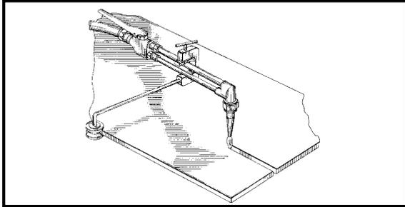
Wheel attachment follows edge of piece to make straight cuts.
