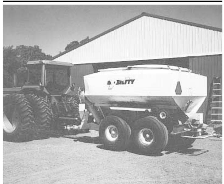
Janikula used a Mobility spinner spreader he bought for \$2,300. Once converted to a soybean seeder, it spreads seed in a 45 to 50-ft. pattern.
