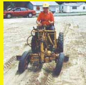
gine. I chose this engine because I had always wanted to hook up one of those old engines to a set of wheels just to see how it would work. The grader has a gearbox of an old 6-speed Wheelhorse garden tractor transaxle. A V-belt off the engine drives a jackshaft which is fitted with a #40 roller chain that powers the transaxle. The tandem drive wheels are 12-in. tires off an old garden tractor.
