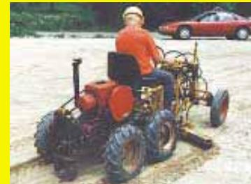
ponents. The blade raises up to 1 ft. off the ground, can be adjusted up to a 45 degree angle either way, and can be moved 1 ft. out to either side with a hydraulic sideshift I rigged up.
