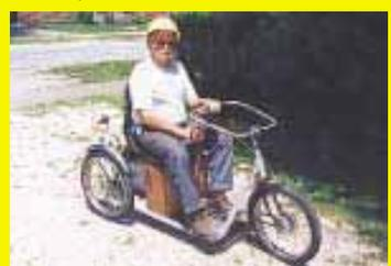
I repowered it with a 3 hp Briggs & Stratton gas engine and a centrifugal clutch like those used on go-carts and motor scooters. Purchased new for the project, the clutch cost more than the tricycle itself.
