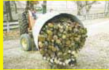
laid the hog feeder on its side and bolted it to the railroad tie and used 2 by 6's on the side of the tines to hold the feeder in place.
