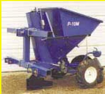
U.S. The 1 and 2-row planters are fully mounted and can be used on tractors with Cat. I or II hitches. Their light weight allows use of a smaller, more maneuverable tractor. The 2-row model adjusts to row spacings from 26 to 36 in. The low height of the 200-lb. capacity seed hopper makes it easy to load from the ground on a pickup bed.
