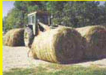
I made a set of double bale forks for the front and back of my Deere 4020 2-WD tractor. They allow me to haul up to four round bales at a time. The front forks mount in place of the bucket on my Farmhand loader bucket. The forks are made to pierce the bale rather than go under it, which results in greater stability and easier unloading. I use the forks in the field to place bales in double rows and later load them onto a truck.
