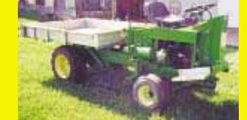
needed something that would haul 1/2 to 3/4 cu. yds. of dirt, yet be small and maneuverable enough that cemeteries would allow it off their roadways to drive between and around gravestones.
