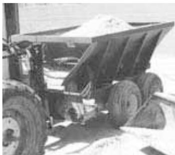
Machine discharges sand 3 to 15 ft. in either direction.
