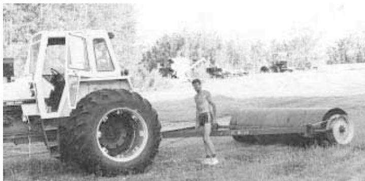
Combine axle hubs mount at either end of the pipe to act as bearings, eliminating the need for a center shaft.
