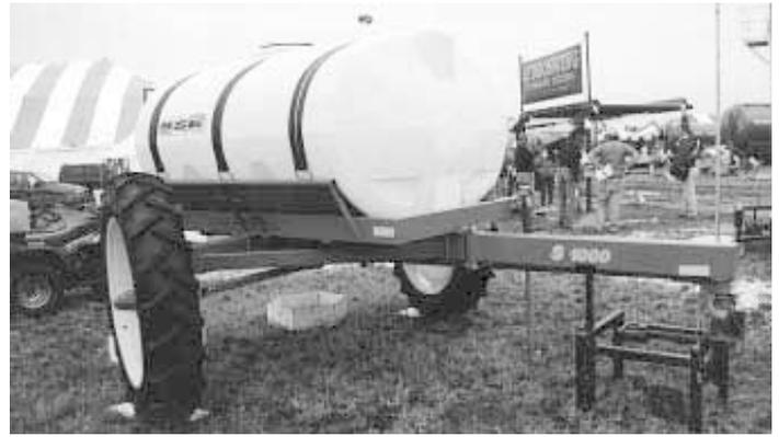
Note how wheels pivot on "steerable" hitch.
