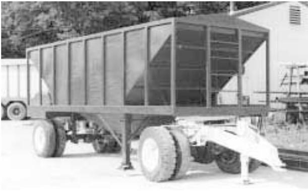
The 20 by 8-ft. wagon was built using the rear axle and jacks off a semi trailer and the front axle and fifth wheel dolly off a semi tractor.
