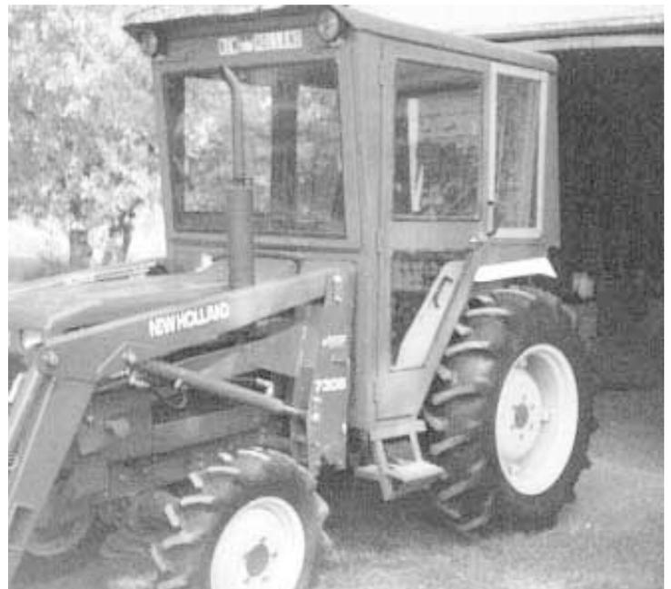
Van Valkenburg had the cab cut down 1 ft. to fit the New Holland tractor.
