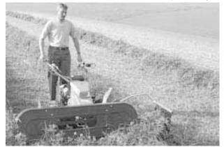
Two-wheeled, hydrostatic unit is equipped with front-mount pto, allowing it to be used with a variety of implements. Driver walks behind and holds onto handlebars.
