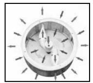
Rotating spray bar inside filter continually sprays a jet of water back through filter screen to keep it clean.
