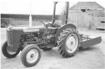
"Smallholder" tractors range from 30 to 55 hp and are based on Massey Ferguson 35 castings. They contain a mix of new and remanufactured parts that keeps cost down.
