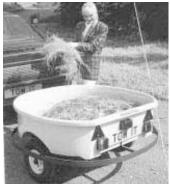
Two-wheeled trailer has a round metal band that goes completely around poly tub.
