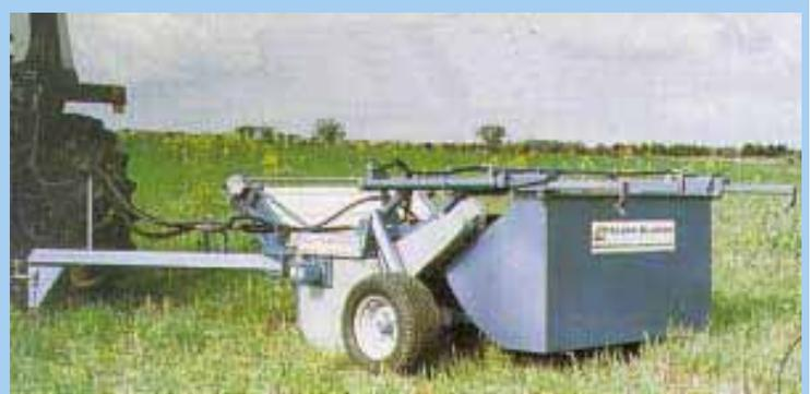
Weeds are fed between a pair of pto-powered rollers which are said to pull 90 percent of weeds in one pass. Working width of the machine is about 5 ft.
