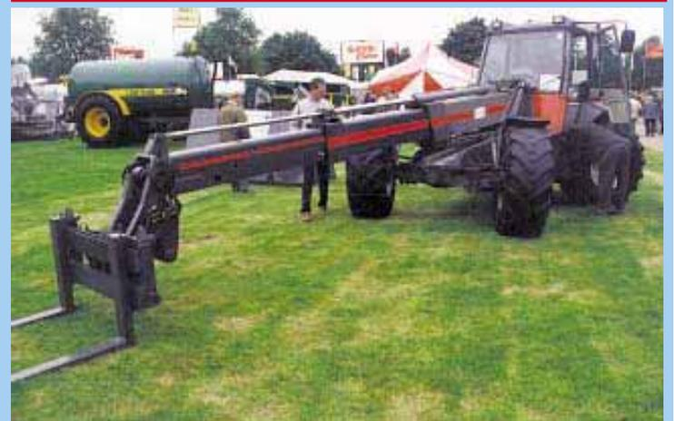
"Teletrak" is equipped with a 3-pt. hitch and drawbar on back and a 3-section, center-mounted boom on front. It can tow loads at up to 25 mph on the highway. "I built it because I wanted a combination of good visibility, towing ability, 4-wheel steering, and 4-WD," says farmer Ken Heard.
