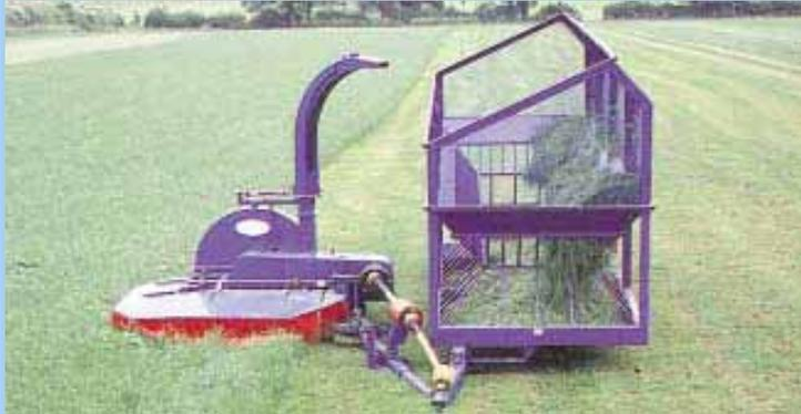
Drum-type mower is pulled alongside a 24-ft. long, 7 1/2-ft. wide feed wagon. Mower is equipped with a swingover drawbar that hooks up to the wagon tongue.
