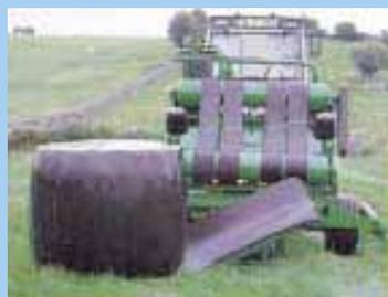
"Side tip" damper allows bales to be gently lowered to ground and tipped on their ends, with no stress to wrapper chassis.
