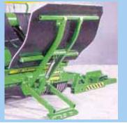
Weeds are fed between a pair of pto-powered rollers which are said to pull 90 percent of weeds in one pass. Working width of the machine is about 5 ft.
