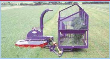
Drum-type mower is pulled alongside a 24-ft. long, 7 1/2-ft. wide feed wagon. Mower is equipped with a swingover drawbar that hooks up to the wagon tongue.
